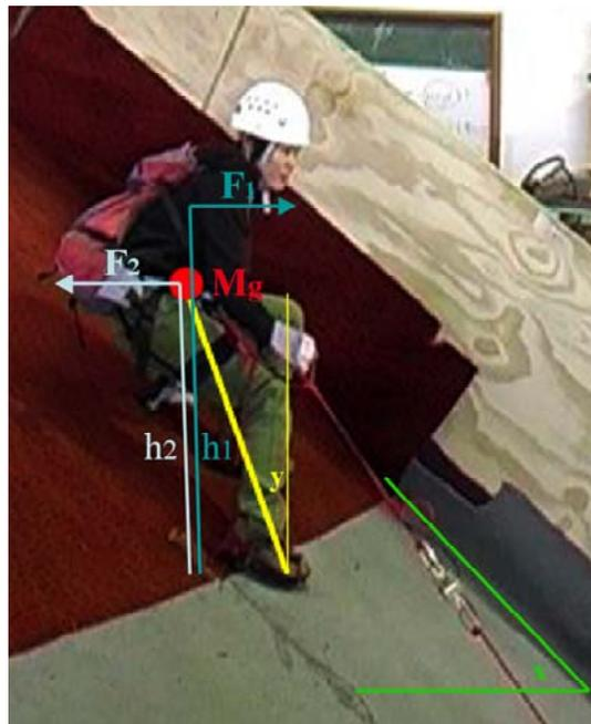
A guide with mass  $M_g$  is reclining with his/her centre of gravity by the angle  $y$  from the vertical. This results in a horizontal force  $F_2$ .
