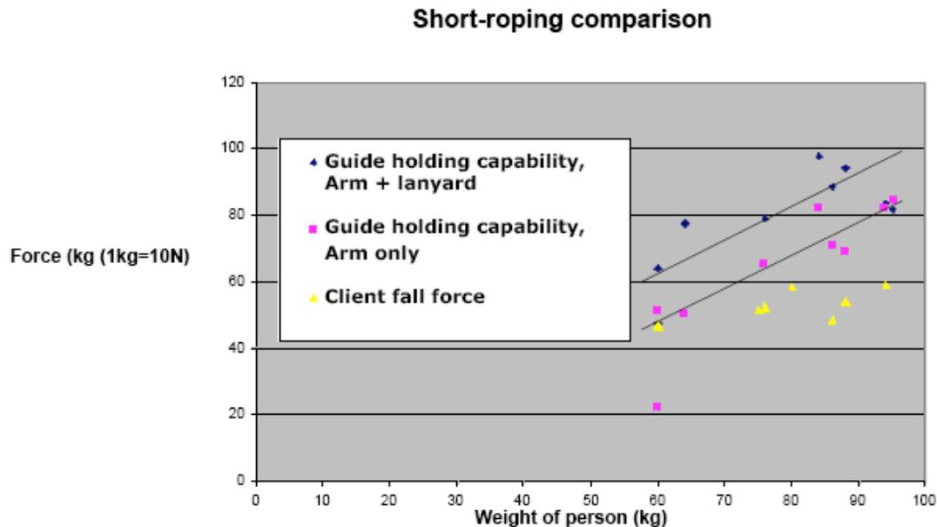
Experiment 2 measured the holding forces of the same guide! The range of measured falling forces might be quite different for a different guide holding the falls, depending on how he/she manages to react to the fall of the client.
